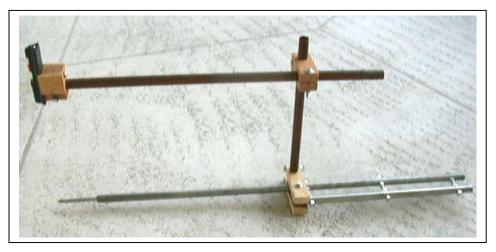
Laser Attachment Mounted on Outrigger
