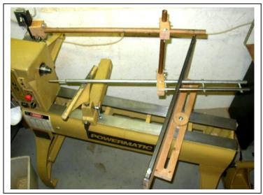
Hollowing Rig Assembled on Lathe
